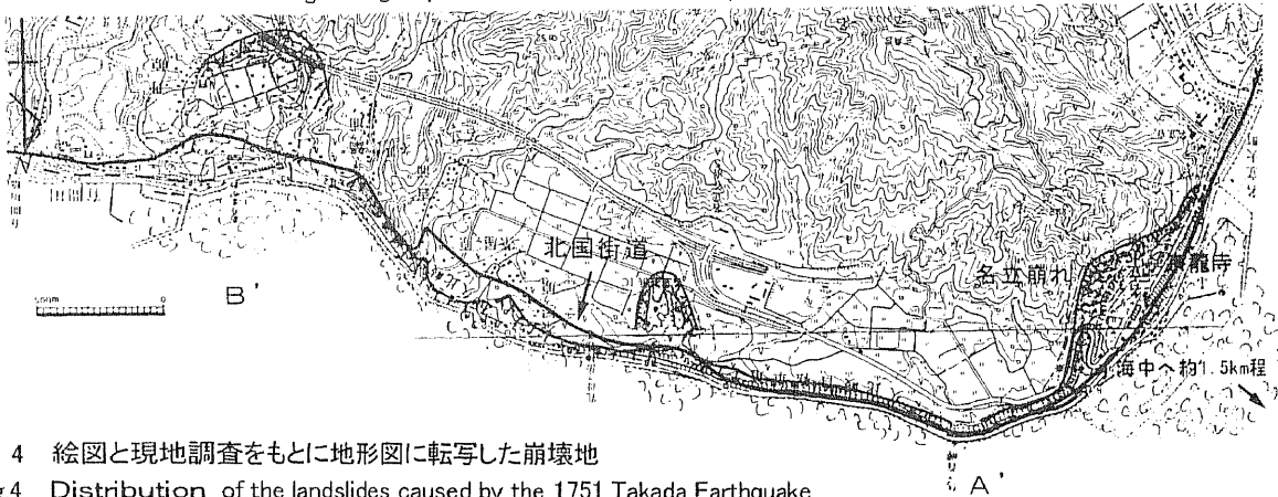
Fig.4 Distribution of the landslides caused by the 1751 Takada Earthquake based on the Big Map and the site exploration
