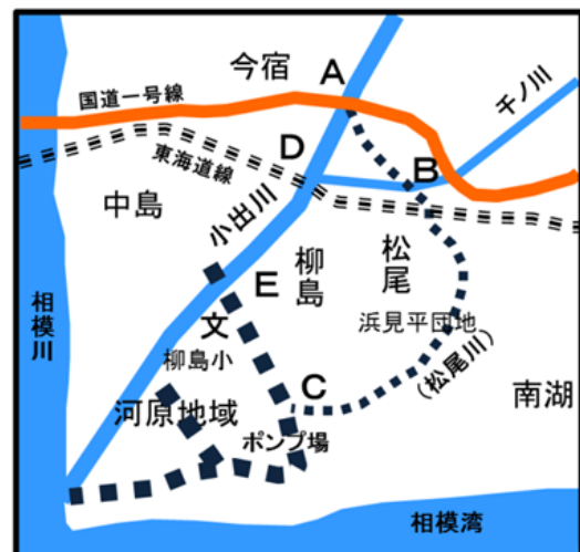
図7 地震前後の柳島付近の河筋の変化 Fig. 7 Change of the course of rivers in Yanagishima area before and after the earthquake.
